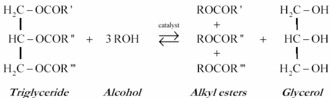
Figure 2. Transesterification process. If methanol is used as the alcohol, fatty acid methyl esters (FAMEs) are obtained.
