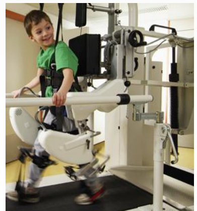
Figure 1: The Lokomat rehabilitation robot improves the efficiency of treadmill training
