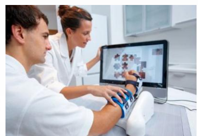
Figure 2: Armaassist, a new advanced rehabilitation robotic platform for Tele-rehabilitation.
